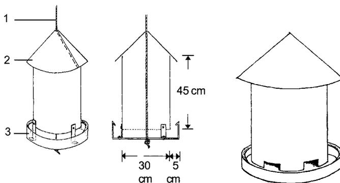
Figure 15: Hanging metal feeder. 1. hanging wire 2. sheet metal cone 3. sheet metal tray
