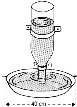
*Figure 16: Water bottle put upside-down into open container*
