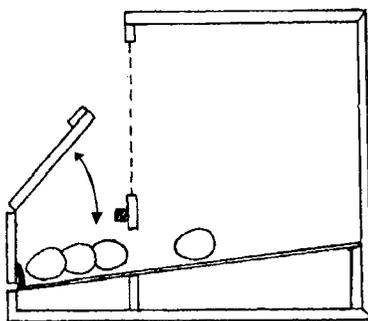
*Figure 23: Cross-section of roll-away nest*
