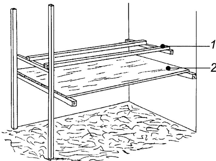
*Figure 17: Perch (1) with dropping board (2)*
