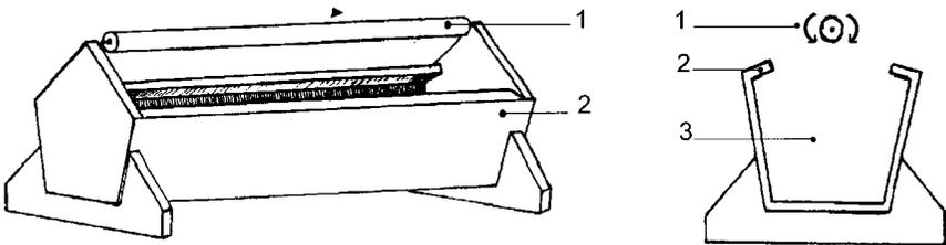
Figure 12: Through feeder on platform. 1. spinner or rotating stick
