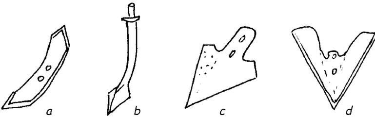
*Figure 36: Several examples of a scarifier tine: (a) The reversible point for scarifying harder soils. (b) The rigid point. (c) The duck-foot point for scarifying lighter soils and general weeding operations. (d) The sweep used for weeding.*
