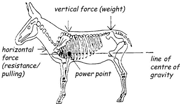
Figure 14: Placement of forces on a donkey's skeleton.
