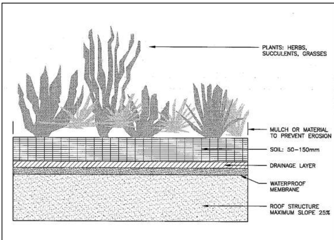
Figure 2: General detail for a low-profile green roof from Waitakere City Council
