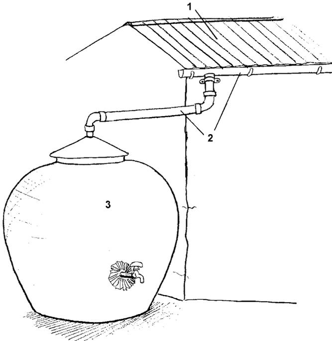
Figure 3: Three basic components of a rainwater harvesting system: catchment (1), delivery system (2), storage reservoir (3)
