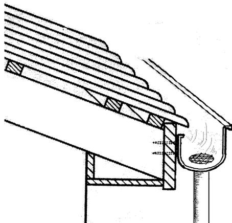
*Figure 25: Coarse filter*
